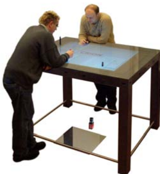
Figure 1: Horizontal interaction space using a back-projection (projector is integrated into the frame of the table, the image is projected onto the tabletop surface via a mirror)
